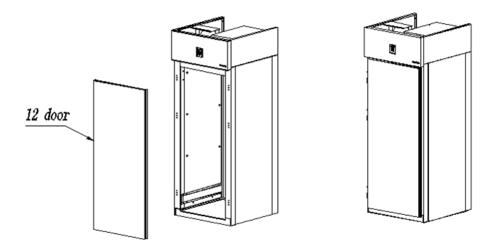
This product must be placed on the horizontal floor to ensure the automatic closure of cabinet doors and proper discharge of condenser water, which is especially important for freezer.
